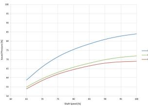
— Conventionally Internal Gear Pump — QXEH Internal Gear Pump — QXEHX Internal Gear Pump
